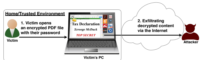
Figure 1: An overview of the attack scenario: The victim opens an encrypted PDF document and unintentionally leaks the decrypted content to an attacker-controlled server. The encrypted PDF file was manipulated by the attacker beforehand, without having the corresponding password.
